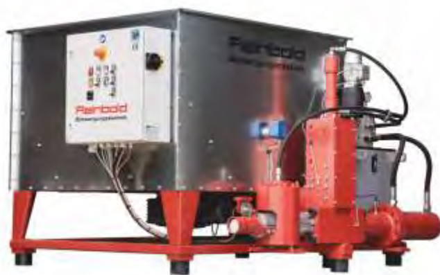
RB 160 with special mechanics for fine dusts
